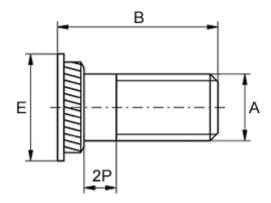
For plate thickness, min = 1.5 Head diameter E = 6 Hole diameter +0.1 = 4.2 Length B = 16 Male thread A = M3x0,5 Min distance to edge = 2.4
